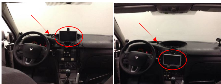
Fig. 2: experimental setting; display in high (left) and low position (right); arrow indicates localization of the remote stimulus for R-DRT
