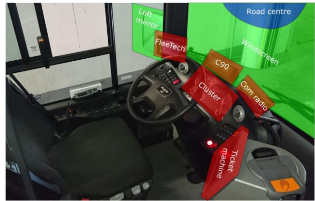
Fig. 1. The cockpit of the bus, including the targets used in the glance analyses.
